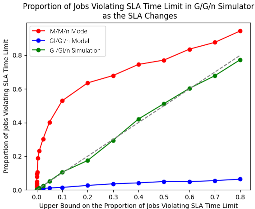
Figure 3.3: The probability of a job waiting for more than 10 seconds in the GI/GI/n environment with the number of service slots calculated by different models as the upper bound on the probability of a job waits for more than 10 seconds changes.
